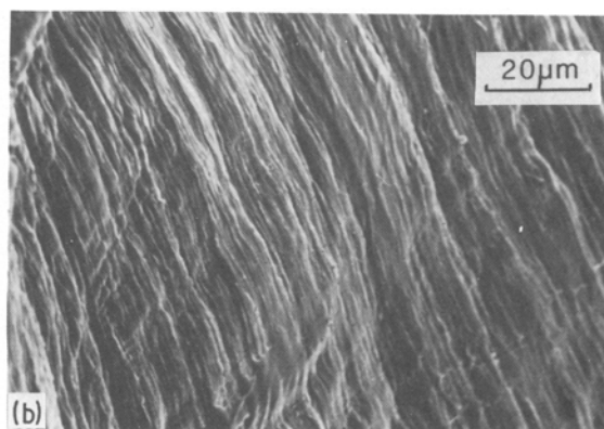
Figure 9 PP weathered in the shade for 3 years and then broken in uniaxial tension: (a) general view of fracture surface; (b) high magnification of part of (a) showing the internal surface exposed by the fracture.
